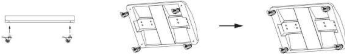
2. Connect the base and the digital poster with provided screws. Tighten all screws with an Allen wrench.
